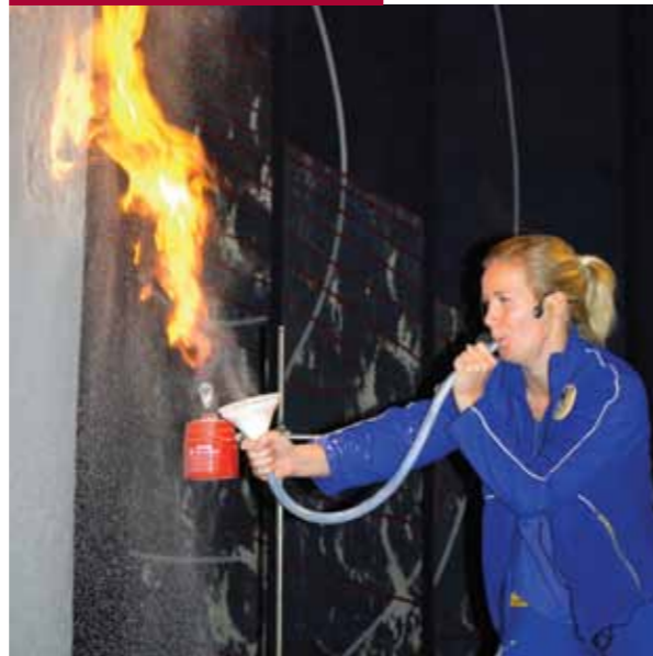
Most people are surprised to learn that ordinary flour can burn with an almost explosive force.
